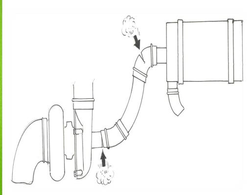
Damaged / Distorted / Ruptured / Loose hoses and/or clamps in the air entry system will allow unfiltered air to be sucked inside by the turbocharger. This will damage the compressor wheel and also force feed the engine with unclean air resulting in damage and failure to the engine as well.
