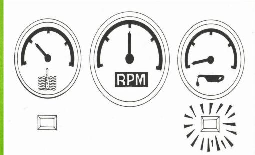
Switch off the engine and contact the service center if the engine oil pressure is low and the warning lamp is glowing.
