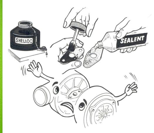
Gasket sealant pastes will block / reduce the oil inlet / outlet passages in the turbocharger.
