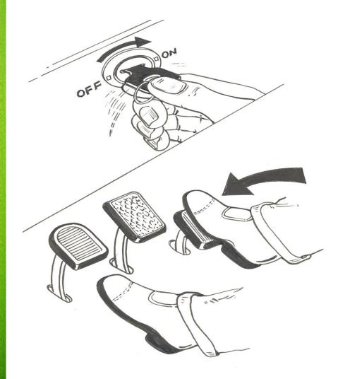
The engine should not be put under full load immediately after start.
