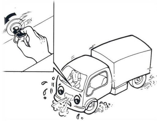
Run the engine without load at high idle for few minutes before the engine is shutoff.
