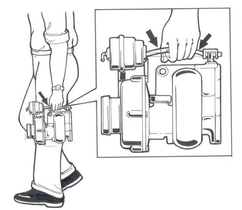
Handle the turbocharger with at most care as it is a very critical component. Safe and proper handling will ensure longer life of your turbocharger.
