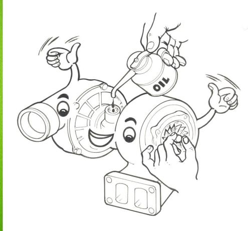
Prime the turbocharger with clean engine oil before fitment after service / repairs.
