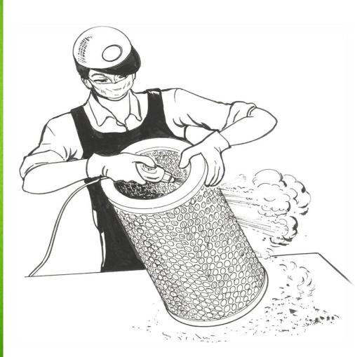
Choked / restricted air system can cause the turbocharger to fail. Clogged air cleaner will restrict the airflow at the turbocharger inlet. This may lead to high exhaust smoke and will also result in seepage of oil from turbocharger into the air intake system.
