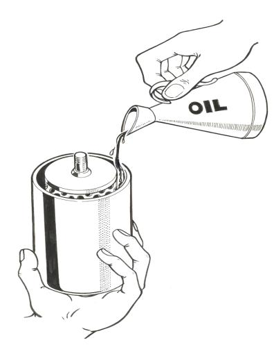
Specified grade engine oil and genuine oil filter should be used and should be changed regularly in accordance with the engine manufacturer's recommendations.
