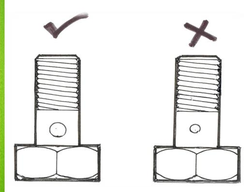
Correct size of banjo bolts ensure that adequate quantity of engine oil is supplied to the turbocharger at adequate pressure.
