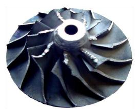
Compressor damage is caused by objects being sucked into the air intake.
