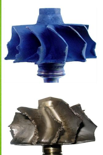
Turbine damage is usually caused by engine components, such as injector tips or valve train parts.
